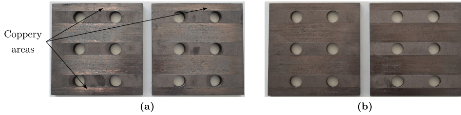
Fig. 11. Surface condition of M1 at the end of the cyclic loading protocol (a) IA-HH and (b) IA for F_{s,exp} = 300\text{kN} .
