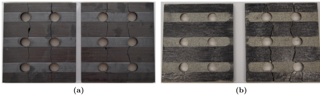
Fig. 15. Fracture patterns of the friction pads (a) M2 and (b) M4 at the end of the loading protocol CA for F_{s,exp} = 300\text{kN} .
